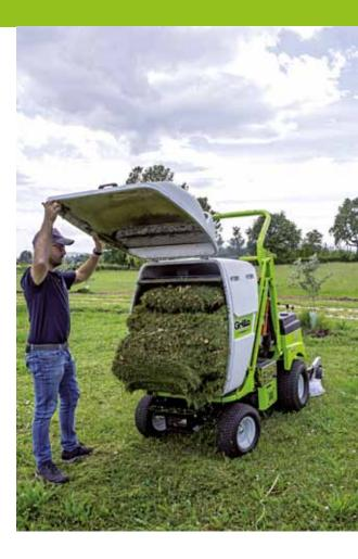
The hydraulic services for raising and tipping the grass collector are operated from the driver's seat by means of convenient levers that make grass discharge and return to the working position extremely smooth and fast.
