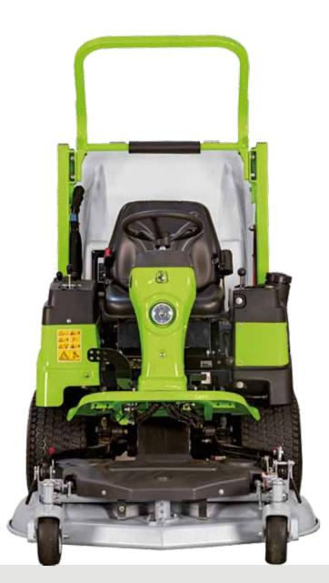
The FD 500 is equipped with an 18 HP 3-cylinder Kubota 722 diesel engine that complies with EC (NRMM) STAGE V (Europe) and EPA Final Tier 4 (USA) standards, mounted on anti-vibration blocks in a very robust monocoque frame, specially designed to protect the mower's components.
