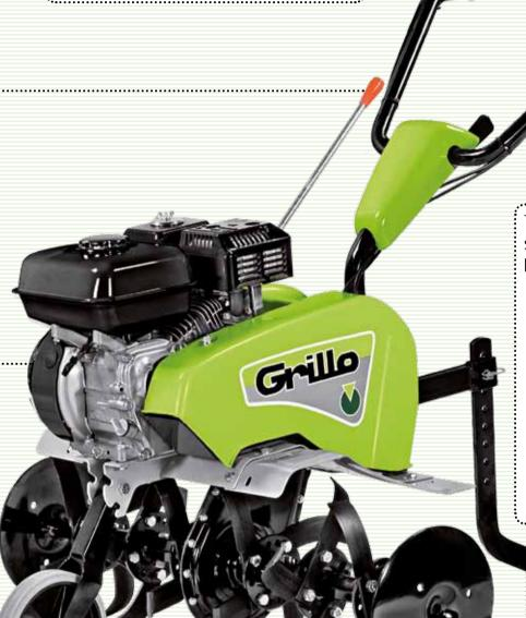
The **handlebar** is adjustable sideways and in height with easy-to-use levers, without need of special tools.
