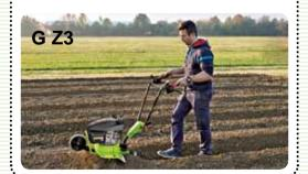
The G Z1 and G Z2 have a standard **tiller** composed of 4 banks of tines 57 cm wide with side discs. Its possible to increase the width up to 80 cm or to shorten it to 35 cm (2 banks). The G Z3 is delivered as standard with an extension kit giving 6 banks of tines.
