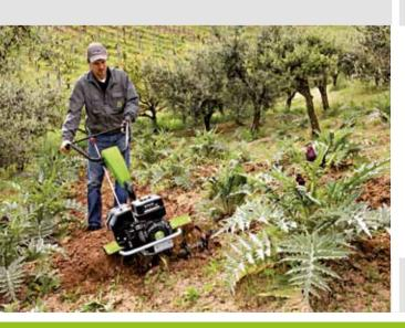
**The front transport wheel** can be lifted and it is optional on 3500 and 11500 models. It can be locked in working or in transport position via a spring device.
